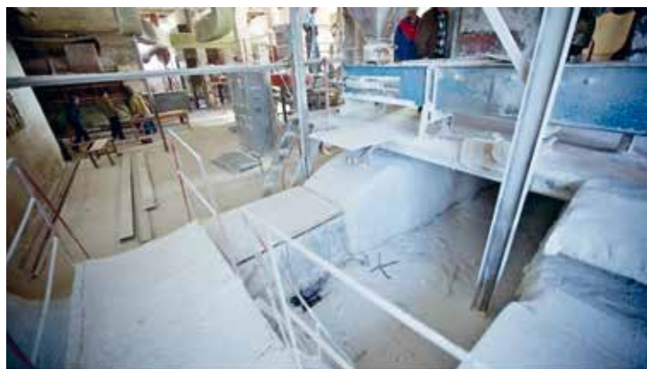
After that, the salt goes to the drying room, where it's dried by means of hot air.
